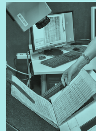
Autographs are photographed with a thermal imaging camera so that watermarks can be seen
